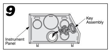
• Insert and snap the key assembly into the hole in the instrument panel.
